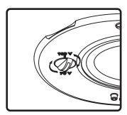
9. Adjust tap switch to proper setting. Switch is preset to the 80hm mode.
